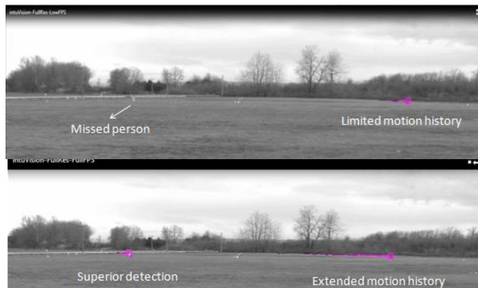
Figure 7: Lower frame rate processing of HD video on a low cost hardware platform misses low contrast small targets (top); GPU enabled full frame rate processing detects and tracks all targets reliably (bottom).
