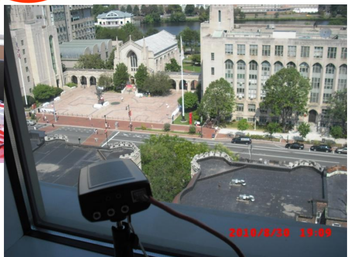
Live camera at AVSS site for real-time processing through intuVision's Panoptes framework.
